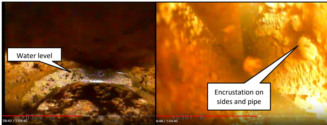
Figure 11: Video survey for Well 4A
